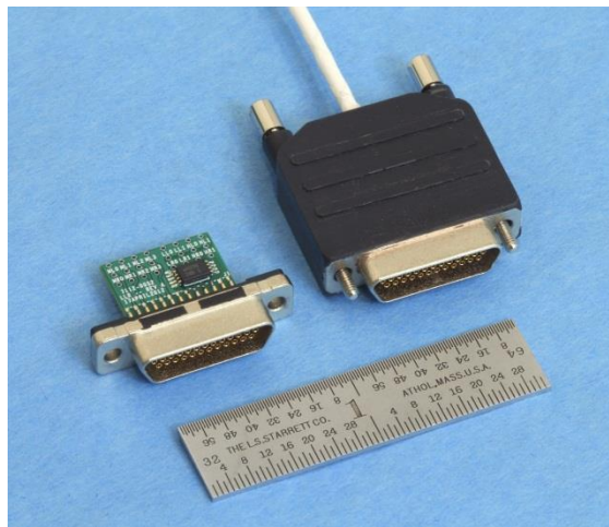
Figure 3. Photographs of the Probe-Side Connector. The left side of the photograph shows the probe circuit board. The single chip visible on the board is a nonvolatile EEPROM for the storing of calibration data. The right side of the photograph shows the probe connector after wiring the probe cable and potting with a hard urethane.
