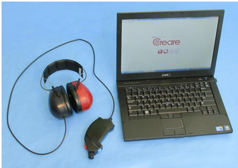
Figure 1. The Clinical Hearing Assessment System. The system consists of a handheld Clinical Hearing Assessment (CHA) module, a calibrated headset, and a PC interface. The CHA can function in wired (USB) or wireless (Bluetooth) modes.
